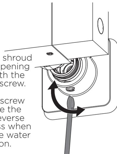
Rotate the shroud until the opening aligns with the isolation screw.
