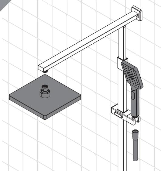
Attach the fixed head, handset (if supplied) and hose (if supplied) to the shower. Ensure the sealing washers are in place if supplied. Turn on the water supply and check all joints and connections for any leaks.
