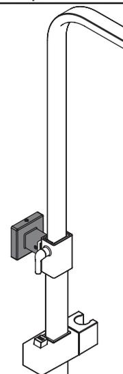
Using a spirit level to ensure the riser is positioned correctly, use the assembled riser to mark the desired position of the bracket.
