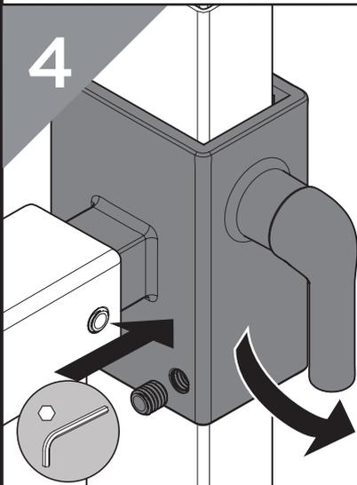
Tighten the grub screws at the back of the bracket to secure the shower arm.
