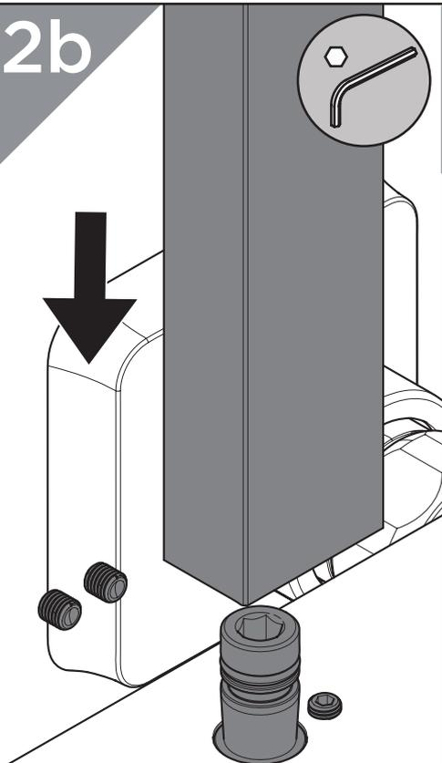
Your riser rail could also be attached via grub screws. Check around the back or sides for grub screw placement.
