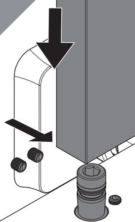
Attach the riser rail to the shower. Check for grub screw(s) placement and secure in place.
