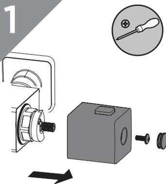
Turn the temperature handle to the max. setting and remove the temperature handle.
