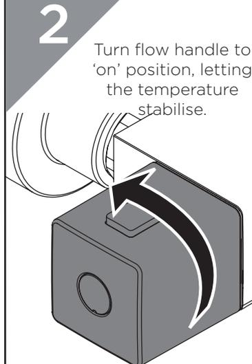
Turn flow handle to 'on' position, letting the temperature stabilise.
