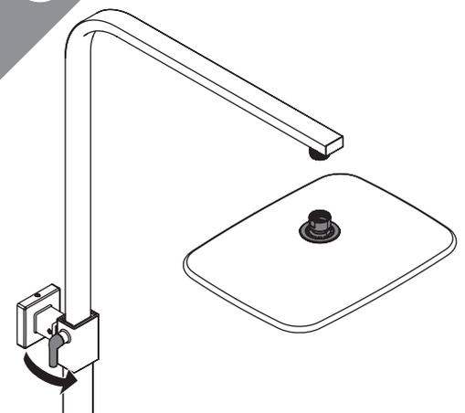
Attach the fixed head. To adjust height of the shower head, see Step 4.
