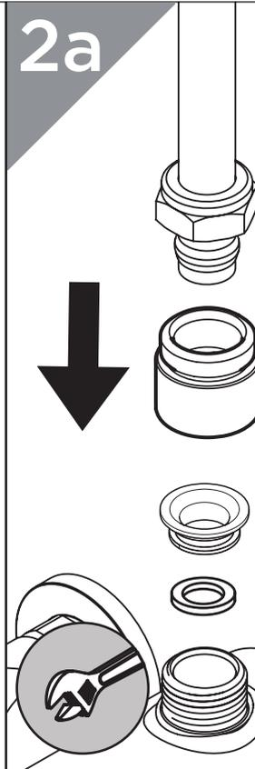
Fit the rigid riser to the top outlet. If attaching directly to a threaded connection, use the threaded adaptor where supplied. Ensure the olive is fitted and tighten the compression nut fully.
