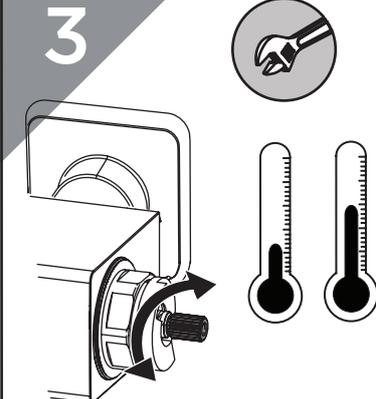
Turn cartridge spindle clockwise to decrease the temperature.
