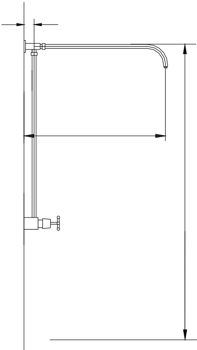
Loosely assemble the riser, making sure it can reach the connection point on your fitting and the bracket will stay flush to the wall.
