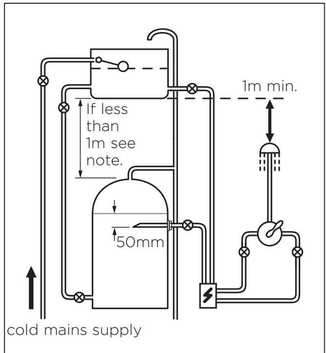
**Key:** ⊗ Isolating Valve    ⋈ Reducing Valve    Ⓞ Shower Valve    ⚡ Pump    ⚒ Essex Flange
