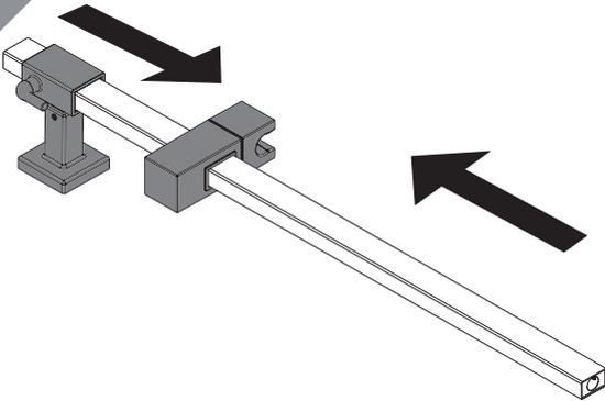
Slide the bracket and slider on to the riser rail.
