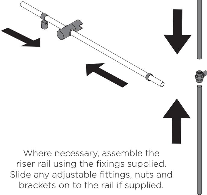
Where necessary, assemble the riser rail using the fixings supplied. Slide any adjustable fittings, nuts and brackets on to the rail if supplied.
