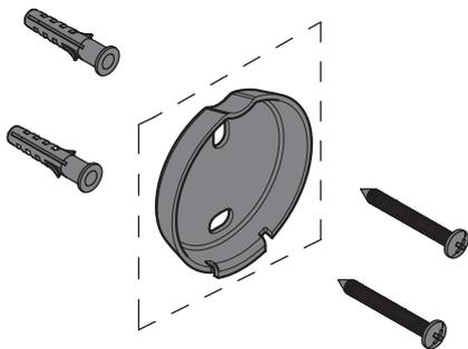
Drill holes. Secure the bracket to the wall.
