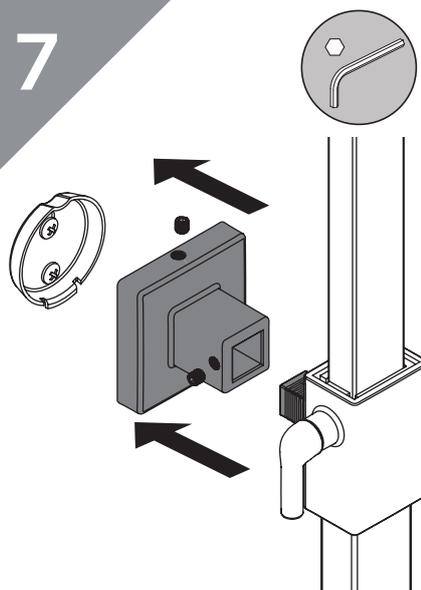
Secure the riser bracket and riser rail.
