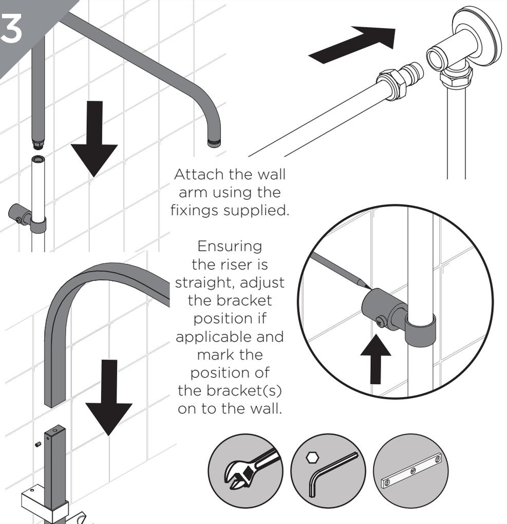
Attach the wall arm using the fixings supplied.
