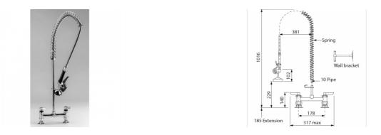
Manufactured from chromium plated brass, both are suited for those locations where there is a need for a thorough rinsing of utensils and crockery in dishwashing areas. F1061 monobloc spray is designed to be fitted into a single taphole behind the bowl whereas the F1062 deck mixer spray fits into taphole centres of 180mm. Both models are supplied complete with spray valve and 150mm wall bracket. Suitable for temperatures up to 130°F.
