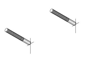
DRILL AND FIT THE WALL PLUGS, THEN SECURE THE BOLTS AS DIRECTED BY THE MANUFACTURERS INSTRUCTIONS
