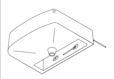
MARK THE POSITION OF THE BASIN AND FIXING HOLES. IF BEING FITTED TO A STUD WALL IT IS RECOMMENDED THAT A BATTEN IS USED FOR SUPPORT WITHIN THE WALL PARTITION.
