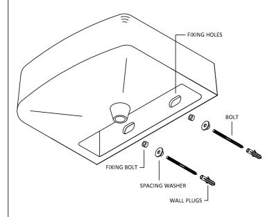
BASIN AND WALL FIXING ANCHOR SET (ANCHOR SET NOT SUPPLIED)
