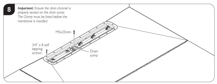
Screw through the drain channel into the drain sump as shown. **Do not over tighten.** Then using an appropriate drill bit, drill through the pre-drilled positions on the top of the drain channel and screw it to the Dec.
