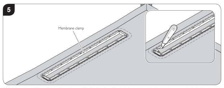
With the membrane laid, use the membrane clamp and find the location of the drain by gently pressing the membrane over the drain channel. Then using the membrane clamp as a guide, cut the membrane flush with the inside edge and remove the centre piece of membrane.
