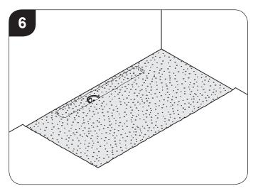
Lay a weak sand cement mix in the excavated hole. **Ensure the mix** is fairly dry. Take care not to get sand and cement in the sump or on the seal.
