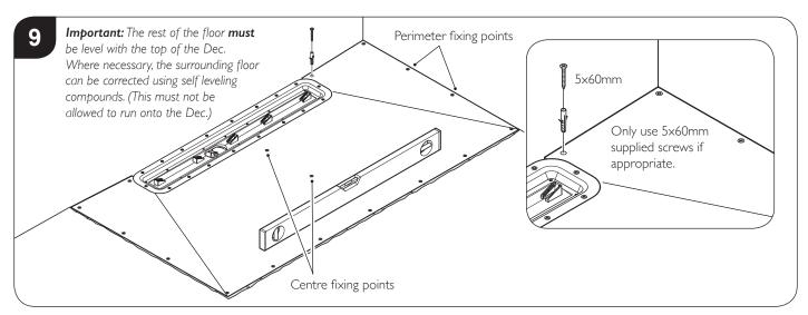
Ensure the Dec is perfectly level, drill and screw it to the concrete below using suitable sized plugs and screws. The Dec should be secured around the perimeter at approx. 200mm intervals and in the centre as shown. **Ensure the Dec does not become distorted when screwing down.** Leave to set over night.
