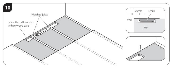
Any joists that cross the drain channel should have notches cut out to take the drain. Re-fix the battens level with the plywood base. Drill and screw the plywood base to the battens below.
