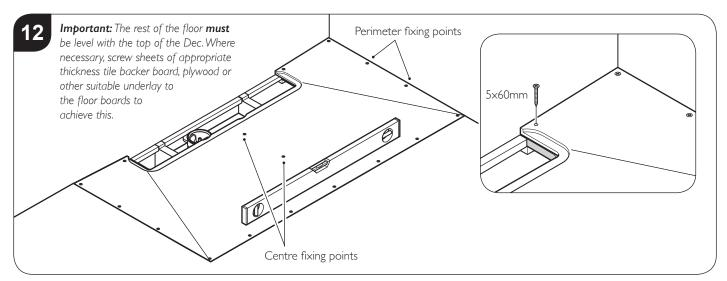
Ensure the Dec is perfectly level, drill and screw it to the plywood below using screws 5x60mm. The Dec should be secured around the perimeter at approx. 200mm intervals and in the centre.
