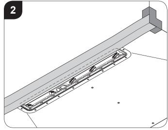
Using the 150mm jointing tape, apply tape along the wall/floor of the 'drain channel edge' so that the tape overlaps 75mm at the wall and 75mm onto the floor.
