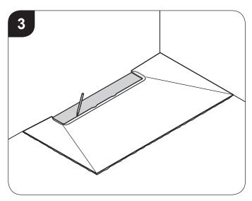
Place the Dec in position and mark a line around the aperture in the Dec, where the drain will fit. Also mark out a 20mm ledge against the wall to support the drain channel.
