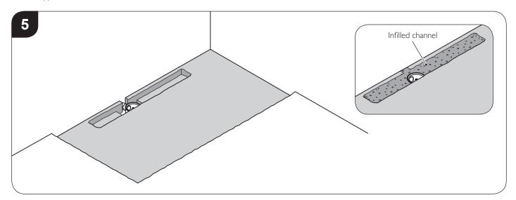
Measure where the drain sump will appear once in position. Place it in the excavated area ensuring the base is sufficiently supported approximately 96mm below the underside of the Dec. Install waste pipework in accordance with current building regulations and connect to the trap using solvent cement. Infill the channelled area for additional support for the drain channel. Take care not to get sand and cement in the sump or on the seal.
