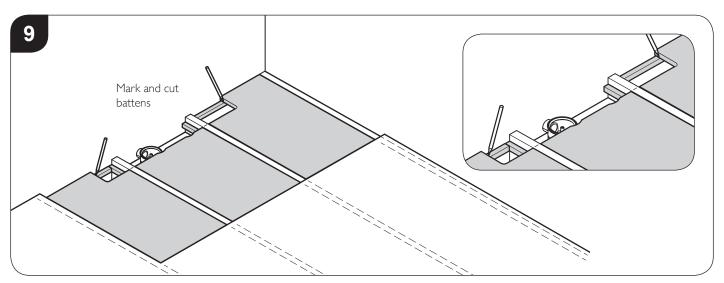
Using a suitable saw cut along the outline previously drawn onto the plywood base. If the lines cross the joists, notch the joists in accordance with current building regulations to a maximum depth of 20mm (this may be reduced if the Dec needs to be packed up). Mark and cut the battens in the opening.
