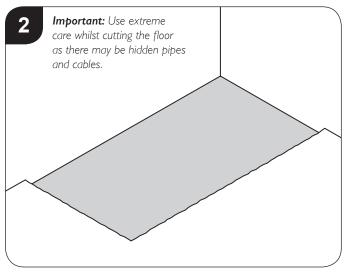
Using a suitable equipment, excavate all the concrete within the marked area to a minimum depth of 35mm.
