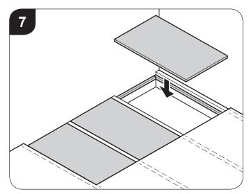
Measure and cut out 18mm plywood panels. Position them, **but do not secure them yet**. Check the panels are level with each other:
