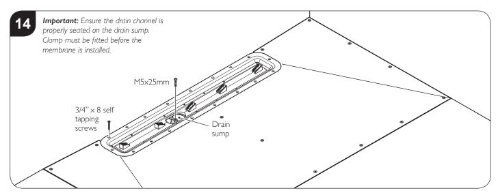
Screw through the drain channel into the drain sump. Do not over tighten.
