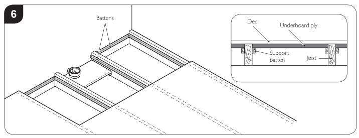
Fix battens to the sides of the joists and noggins. To provide a flat and level base for the Dec, the battens must be fixed 18mm below the top of the joists to allow for the thickness of the plywood.
