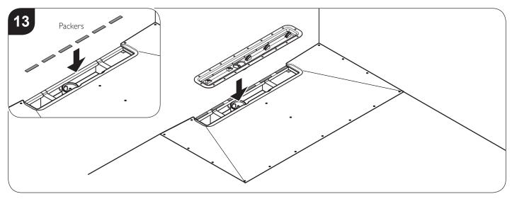
Place packers along the 'wall' batten to support the drain channel. Position the drain channel into the Dec.
