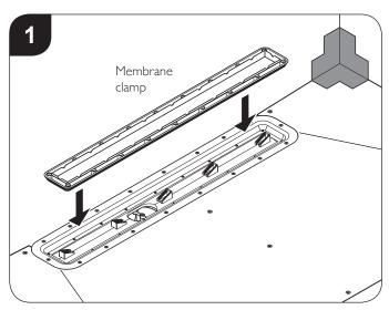
Place the membrane clamp into position on the drain channel (do not fix yet).
