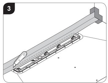
Carefully cut the joining tape following the gap between the drain channel and the membrane clamp (using the outer edge of the membrane clamp as a guide).
