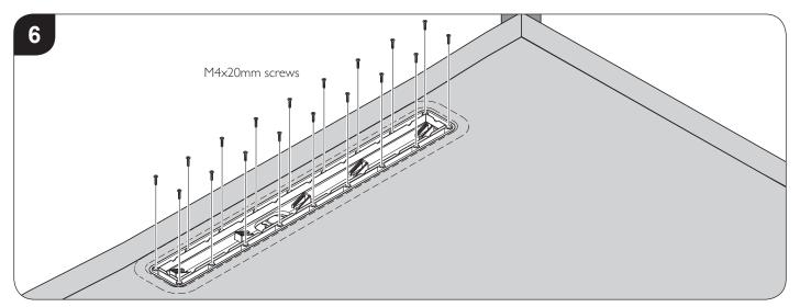
The membrane clamp should be carefully pressed into position to allow the membrane to stretch over the drain channel, once the membrane has begun to stretch into place, gradually tighten the screws. **The clamp must be lowered evenly into place. Do not use power tools.**
