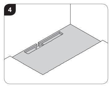
Remove enough concrete for the installation of a waste pipe and shower trap/Linear drain channel.
