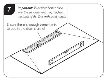
Position the Dec onto the weak sand/cement mix ensuring it is flush with the surrounding floor and perfectly level. **This is very important for correct drainage from the Dec.** If not level, pack more weak sand/cement mix under the Dec.
