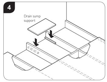
A support 96mm below the level of the bottom of the Dec should be fitted, this is for the drain sump to rest on.
