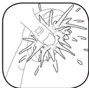
1. To break away scale deposits on a daily basis simply rub your thumb over the surface whilst the shower is running.
