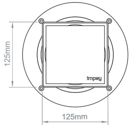
**Pumped Drain;** 22mm outlet
