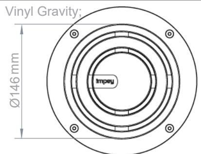
**Slimline Drain;** Un-trapped waterless floor drain
