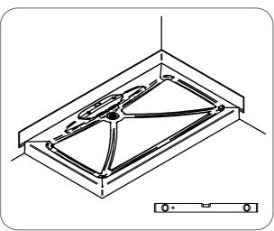
Place the tray in position again and check that it is level on all 4 sides. If it is not pack it up as necessary.
