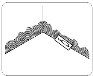
**Q** Apply tile adhesive to wall in upstand area.
