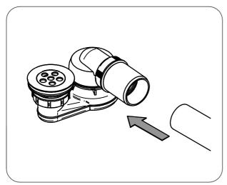
Fit the waste pipe to the trap using solvent weld and route the pipe under the tray so that it exits through the previously drilled hole.
