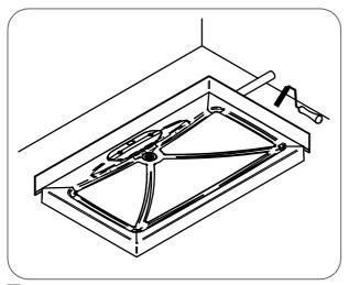
7 Using a roller press tape into place firmly. Ensure air gaps or creases are removed.
