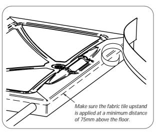
Remove first 10cm of release paper in one smooth action, then continue removing the paper while carefully applying tape with other hand until required edge is covered. Do not stretch as you apply.
