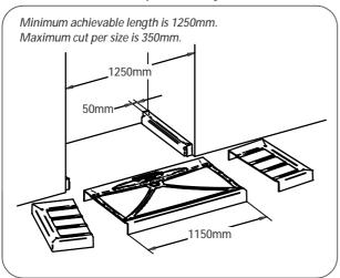
Minimum achievable length is 1250mm, cutting both sides of the tray and using both left and right hand end caps. The length of the tray after it has been cut will equal the width of the trecess reduced by 100mm (50mm for each endcap). Follow steps 3-4 to finish the installation.
