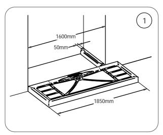
Measure the area where the tray will be installed. Place the endcap in the desired location. The length of the tray after it has been cut will equal the width of the recess reduced by 50mm (size of the endcap). Maximum cut per side is 350mm.
