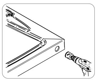
4 Using a 45mm-50mm hole saw, drill the waste pipe hole in the side of the tray.
