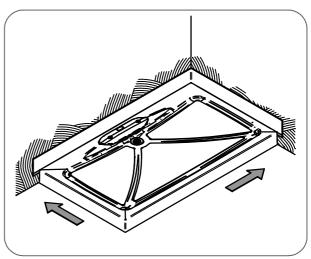
10 Put the tray in position and press the upstand into tile adhesive ensuring there are no air gaps. Allow 24 hours before exposing to water.
