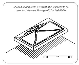
Determine which corner the tray is to be fitted into. This will establish which edges the fabric tile upstand will be attached to.
