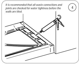
Follow the fixing instructions in the main installation guide ensuring the tray is level. With the tray in position, carefully seal the joint between the tray and end cap with silicone sealant.
