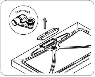
2 Remove the access cover to enable better access for fitting the trap. Determine which direction the waste pipe will run and twist the swivel outlet of the trap in the appropriate direction.
