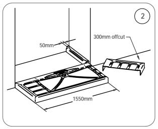
Trim the tray using a fine blade saw, exercising extreme care not to damage or chip the finish of the tray.
