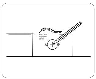
3 Using apropriate waste hole drilling locations template, mark the location of the waste hole. Refer to the drilling guide on page 6 and waste hole drilling locations template on page 7.
