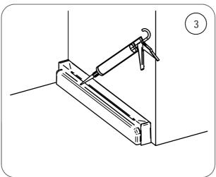
Apply a generous bead of silicone sealant to the support face of the end cap, connect the waste trap and pipe to the tray, then apply silicone sealant to the cut edge of the shower tray to prevent ingress of moisture. Place the end cap onto the tray.
