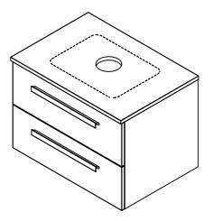
CUT-OUT THE WASTE ALLOWING FOR ACCESS (APPROX 120mm DIAMETER) MAKING SURE THE CUT OUT IS NOT VISIBLE WHEN THE BASIN IS IN PLACE. ALSO CUT OUT FOR THE TAP AND CONNECTIONS IF REQUIRED. ENSURE ALL CUT EDGES ARE SEALED AGAINST WATER INGRESS.
