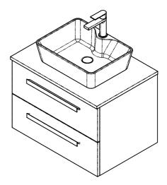
PLACE THE BASIN IN POSITION ON THE WORK SURFACE AND PRESS DOWN TO MAKE A SEAL. CLEAN OFF ANY EXCESS SEALANT (FOLLOW THE MANUFACTURERS INSTRUCTION REGARDING CURE TIME) FINALLY, MAKE ALL SERVICE CONNECTIONS.
