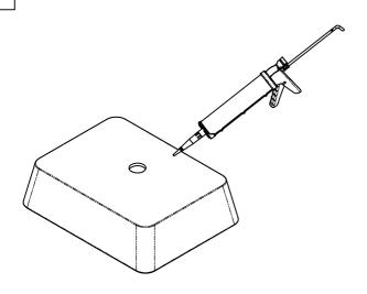
FIT THE BASIN WASTE, MAKING SURE THERE'S A GOOD SEAL. FIT ANY BRASSWARE AND CONNECTIONS IF REQUIRED AT THIS POINT. APPLY A BEAD OF SILICONE AROUND THE BASE OF THE BASIN THAT WILL BE IN CONTACT WITH THE WORKTOP.
