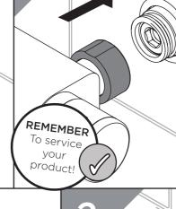
Secure the isolator onto the backplate ensuring the olive is positioned over the
