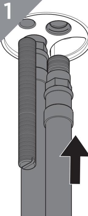
Screw in the flexible tails by hand. **DO NOT OVERTIGHTEN.**
