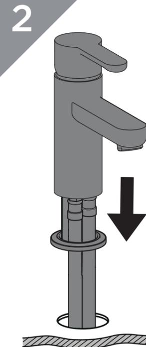
Fit the tap to the basin, ensuring the base washer is in place.
