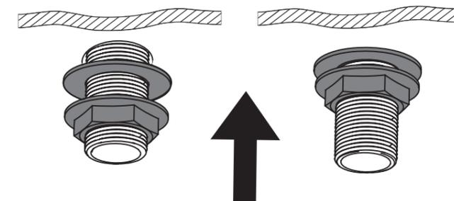
Secure the taps to the bath by using the washer and metal backnut below the bath.
