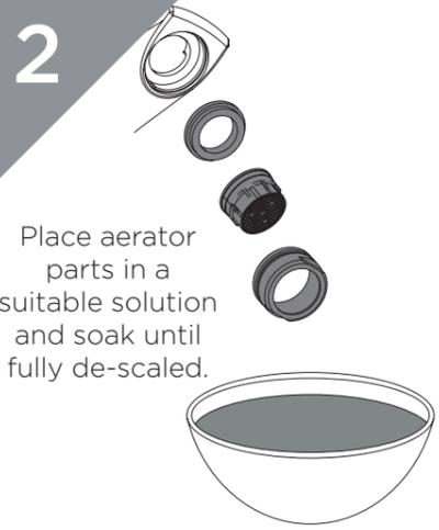
Place aerator parts in a suitable solution and soak until fully de-scaled.
