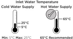
The inlet hot water must be at least 10°C above the required blend temperature.
