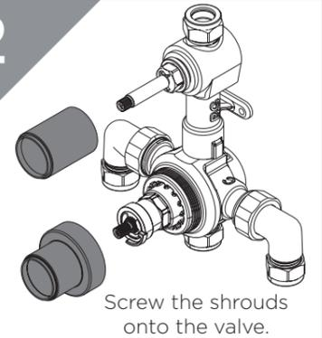
Screw the shrouds onto the valve.
