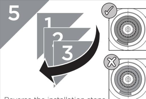
5 Reverse the installation steps, ensuring the temperature stop is aligned correctly.
