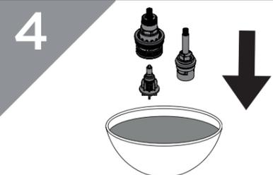
4 Remove any O-rings and soak all components in de-scaler and wash off in clean water. Examine all seals and replace if needed. Use WRAS approved silicon based grease on all seals.
