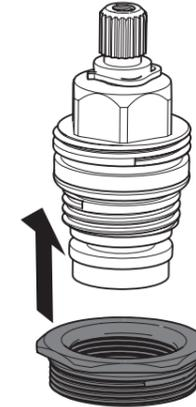
If the thread in body is larger then fit the 1/2" 1010 tap insert and follow assembly chart on 1/2" 1010 section.
