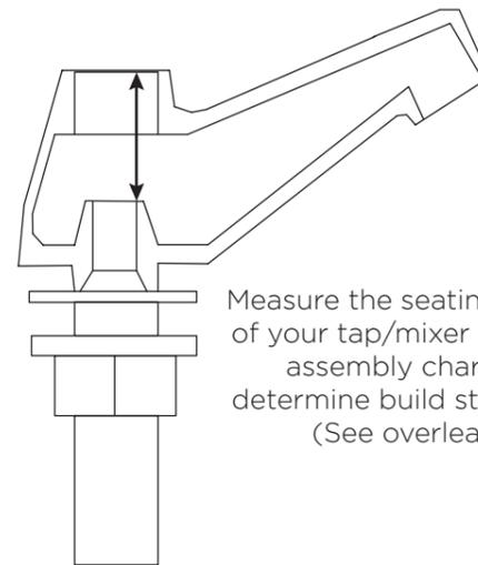
Measure the seating depth of your tap/mixer and see assembly chart to determine build structure. (See overleaf)
