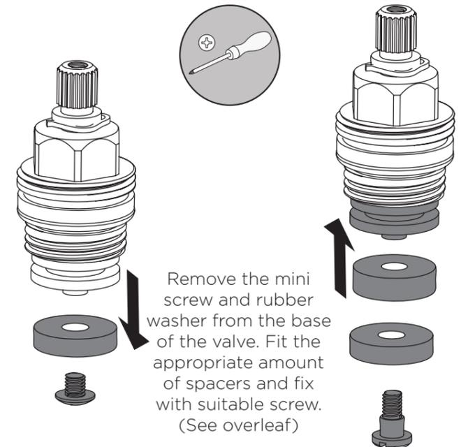
Remove the mini screw and rubber washer from the base of the valve. Fit the appropriate amount of spacers and fix with suitable screw. (See overleaf)
