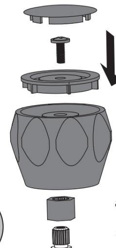
Fit the spline adaptor and handle to the valve. Fit insert indicator, secure with screw and cap.
