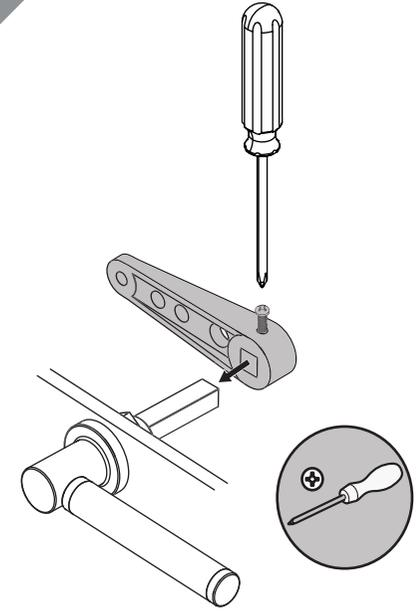
Attach the cistern lever arm and tighten with the locking nut.
