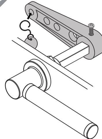
Hook the clip from the flush mechanism on to the adjacent hole of the arm. The handle should approximately sit between 2-3 O Clock.
