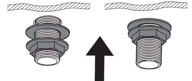
Secure the taps to the basin by using the washer and metal backnut below the basin.
