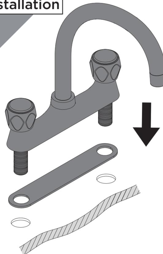
Feed the tap body through the tap holes, ensuring the gasket washer is in place.
