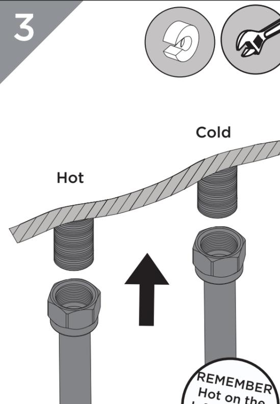
Connect the hot and cold water supplies to the threaded tails.
