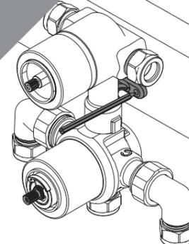
Install suitable batons (if required) into the cavity. Mark the position of the valve; drill and plug holes to suit.
