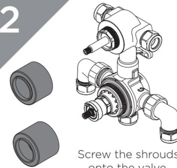
Screw the shrouds onto the valve.
