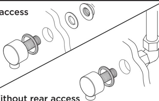
Follow Step 6 in the Installation Steps, fitting a 1/2" female connection at the hole in the wall (not supplied).
