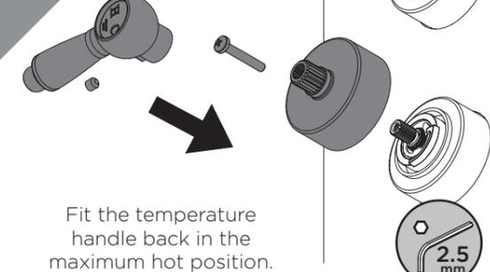
Fit the temperature handle back in the maximum hot position.
