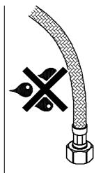
The braiding on the flexible hose must not be in contact with anything else, for example chemicals, internal or external room walls or dissimilar metals or materials or sharp objects.
