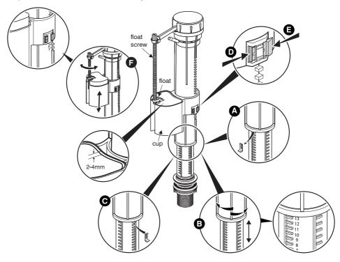
Connect the water supply to the inlet valve. Turn on the water supply and allow the cistern to fill. Adjust the float on the inlet valve so that the valve stops the flow of water when the water reaches the waterline marked in the cistern. Check for leaks.
